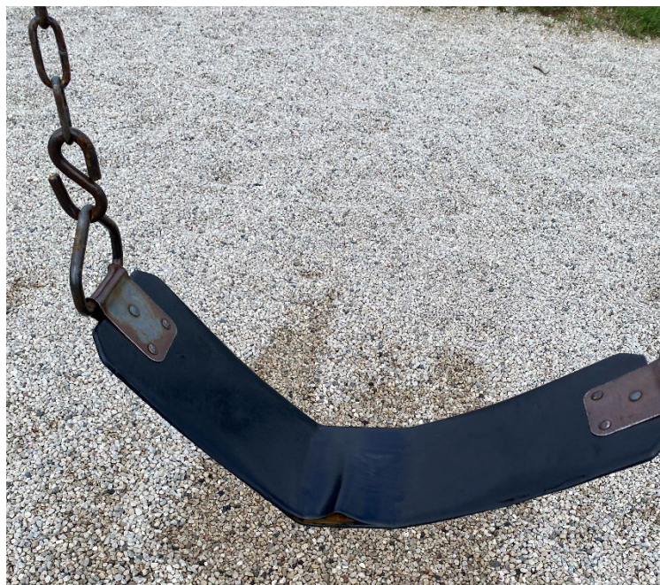
Figure 58: Broken swing seats on back swing set.
